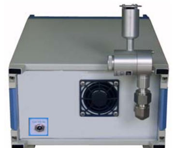
IQM 60 rear view of cooling fan, 12VDC power connection, PM10 or PM2.5 sharp cut cyclone and isokinetic inlet for an optional Particle Monitor
